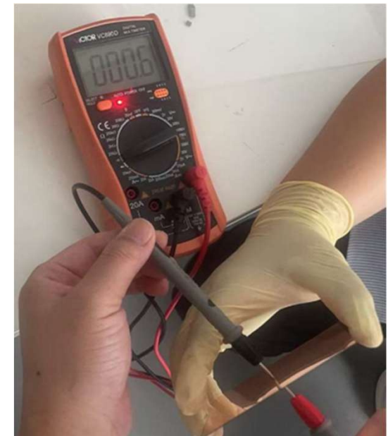
Sputter後用萬用表測量電阻值0.6MΩ
